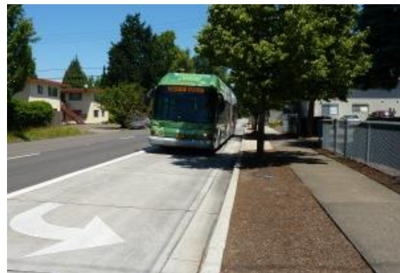
BAT lanes are bus-only lanes that may be used by right-turning vehicles.
